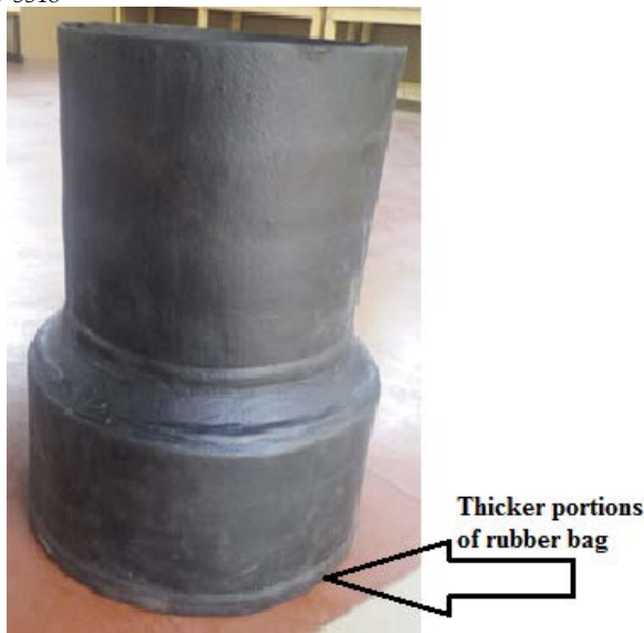
Fig-6 More thicker portions observed near bottom of rubber bag
