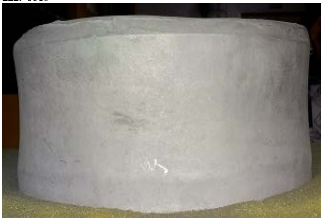
Fig-5. Roll pressed after changing the rubber bag material to natural rubber with uniform thickness.
