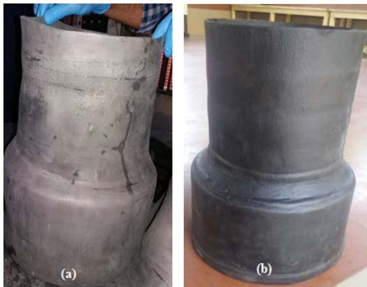
Fig 4 (a) Rubber bag madeup of PVC, (b) rubber bag madeup of natural rubber with uniform thickness
